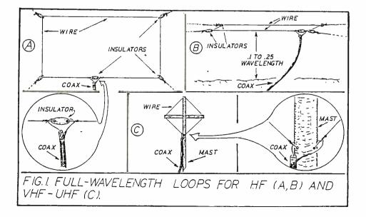
each insulator. For VHF loops cut the cross arms to length, make center notches in the arms, and put holes in the arm ends for the wire. Glue the arms into a cross and run the wire through the holes in the arm tips.
